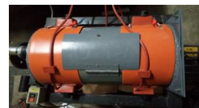
Fig. 2. Container with heater pads
