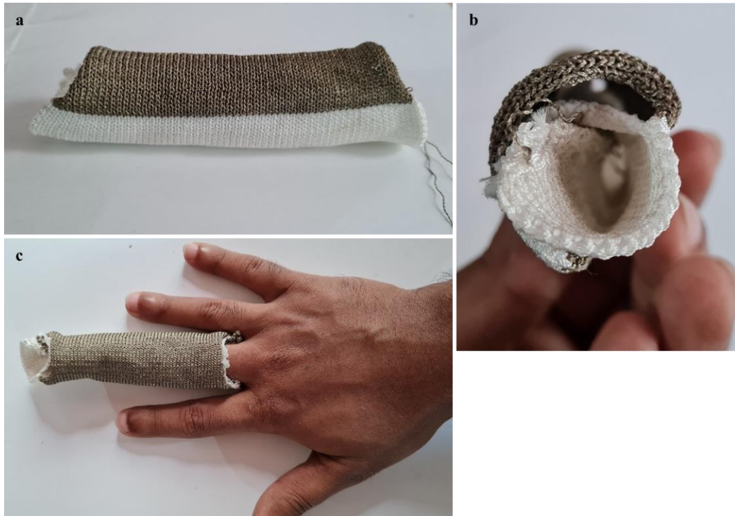
Figure 4.5: TENG sensor. (a) Top view. (b) Side view. (c) TENG sensor worn to a finger
