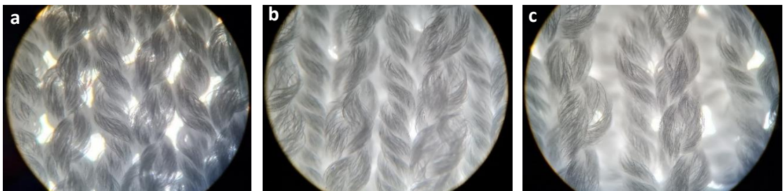
Figure 5.10: Microscopic images of (a) single jersey, (b) Interlock, (c) rib structures when stitch density is constant.
