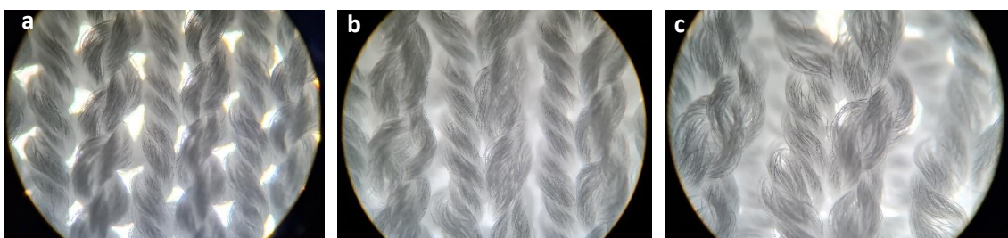
Figure 5.11: Microscopic images of (a) single jersey, (b) Interlock, (c) rib structures when loop length and yarn counts are constant.
