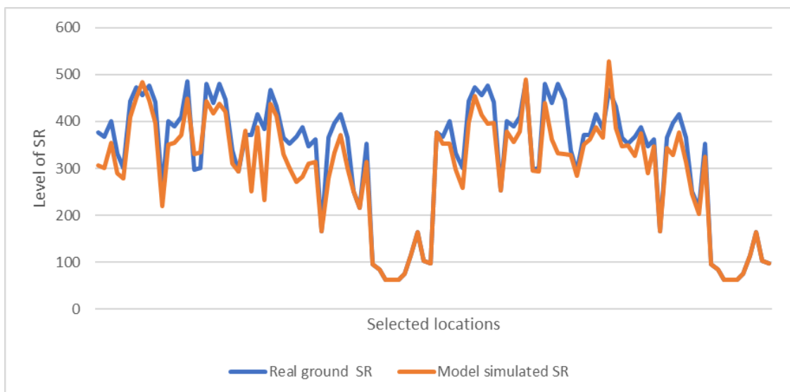
Figure 23: Differences between model results and real-world data on surface runoff – sub catchment level
