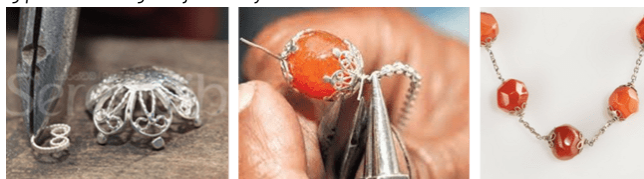
Figure 6 Assembling process of Agasti jewellery
