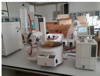
Figure 2 Evaporating DSW using Rotary Evaporator
