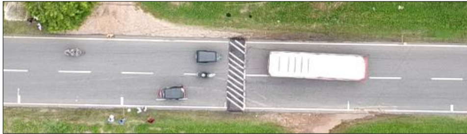
Figure 1. Drone view of 75mm height hump located at the 10 th kilometer post on B-300 Road
