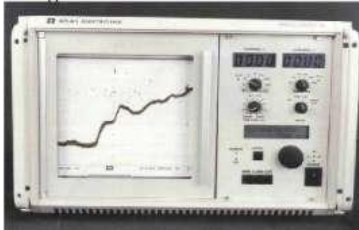
Example Figure 3: A typical echo sounder to drown topography (Arnoldo, 1999)
