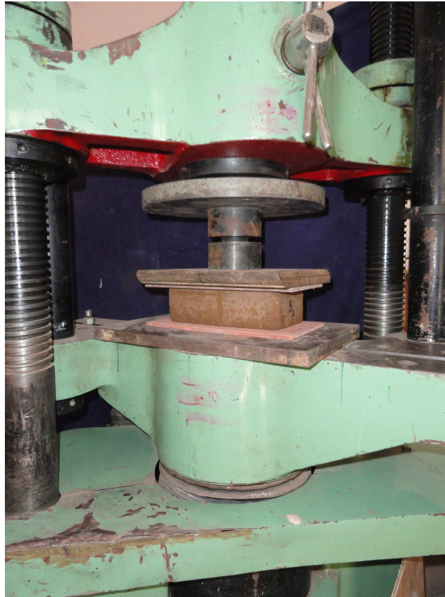
Fig. 3 – Brick under wet compressive strength test
