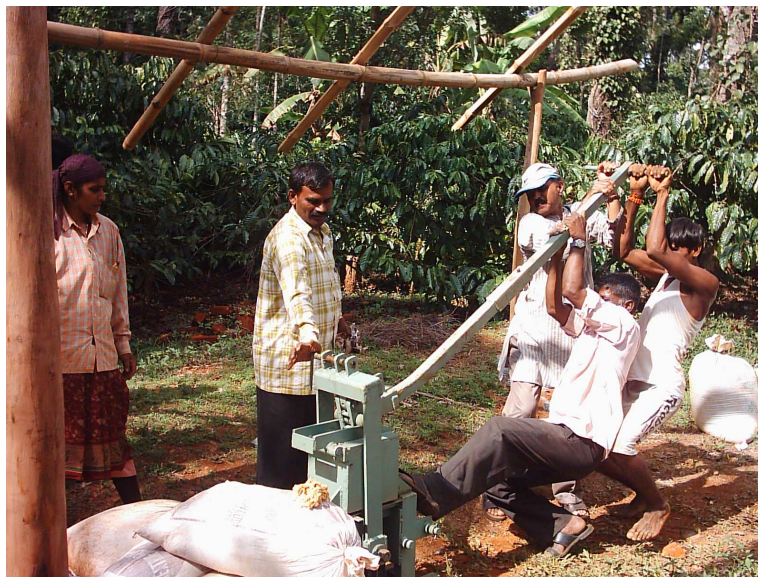
Fig. 2 – Production of compacted SMB using manual press
