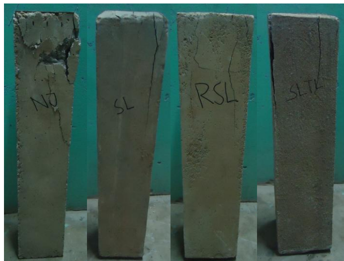
Figure 5: Typical failure pattern of tested specimens.
