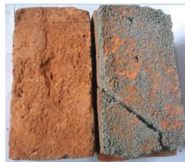
Figure 1: Rupture modes in couplet specimens with machine made bricks Figure 2: Rupture modes in couplet specimens with hand-made bricks
