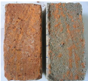
Figure 1: Rupture modes in couplet specimens with machine made bricks Figure 2: Rupture modes in couplet specimens with hand-made bricks
